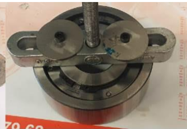
open puller with M5X35 turned into Backstop threaded holes M5 , rotated center spindle into the shaft
